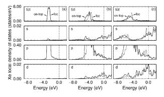
FIG. 2. Local density of states for Xe on Pt(111) for different vertical positions (Z) of Xe: (a) Z = 4.53 Å; (b) Z = 3.07 Å (equilibrium Xe position); (c) Z = 2.70 Å.
