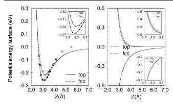
FIG. 4. Left panel: Calculated binding energies of Xe on Pt(111) for the on-top and fcc sites as a function of distance from the surface. The filled and open circles indicate DFT-LDA data. Right panel: decomposition into repulsive and attractive contributions (see text). Z = 0 is the center of the top layer.
