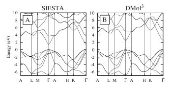
FIG. 1. Band structure of wurtzite GaN calculated using (A) SIESTA and (B) DMOL<sup>3</sup>.
