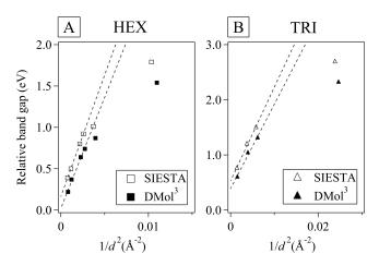
FIG. 12. Relative band gap as a function of  $1/d^2$  for saturated (A) hexagonal and (B) triangular nanowires, where *d* is the nanowire diameter. The dashed lines indicate the linear regions for each of the data sets. "Hex" and "Tri" represent "hexagonal" and "triangular," respectively. Band gaps are relative to the calculated bulk GaN band gap.
