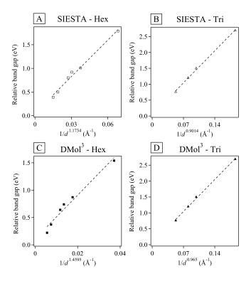
FIG. 11. Relative band gap as a function of  $1/d^{x}$  for saturated (A) hexagonal and (B) triangular nanowires with SIESTA, and saturated (C) hexagonal and (D) triangular nanowires with DMOL<sup>3</sup>, where *d* is the nanowire diameter. The dashed lines indicate the linear regions for each of the data sets. "Hex" and "Tri" represent "hexagonal" and "triangular," respectively. Band gaps are relative to the calculated bulk GaN band gap.
