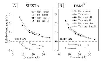
FIG. 10. Relative band gap as a function of nanowire diameter as obtained using the (A) SIESTA and (B) DMOL<sup>3</sup> codes. Band gaps are relative to the calculated bulk GaN band gap. "Hex" and "Tri" represent "hexagonal" and "triangular," respectively, and "unsat," "sat," and "sat-frac. H" represent "unsaturated," "saturated," and "saturated with fractional charge hydrogen," respectively.
