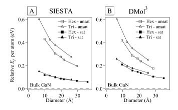
FIG. 13. Relative heat of formation (per atom) as a function of nanowire diameter for unsaturated and saturated nanowires in the [0001] direction, from (A) SIESTA and (B) DMOL<sup>3</sup>. Energies are relative to the heat of formation (per atom) of bulk GaN. "Hex" and "Tri" represent "hexagonal" and "triangular," respectively, and "unsat" and "sat" represent "unsaturated" and "saturated," respectively.
