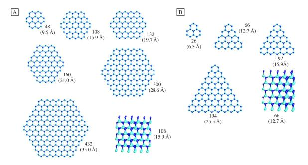
FIG. 2. (Color online) Nanowires in the [0001] direction that have (A) hexagonal and (B) triangular shaped cross sections, viewed along the wire direction, with perspective views of the 108 and 66 atom nanowires included. The number of atoms used in the calculations for each nanowire, and the diameter (in parentheses) are also labeled. Nitrogen and gallium atoms are indicated by the dark (blue) and light (aqua) spheres, respectively.
