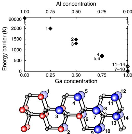
FIG. 4 (color online). Calculated relative formation energies, K, as a function of the cation concentration  $x$  in the Cr-doped graded  $\text{Al}_{1-x}\text{Ga}_x\text{N}/\text{GaN}$  (0001) heterostructures and geometry of the corresponding supercell. The numbers on the graph correspond to those in the supercell and denote the Ga site locations substituted with a Cr atom.
